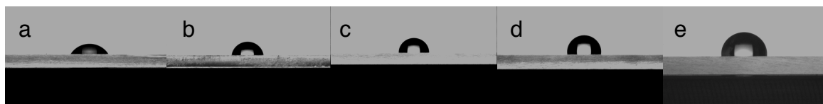
Figure 2-5: WCAs of droplets on a) HDDA b) 1.5 wt% of 2.1[NTf 2 ] c) 1.5 wt% of 2.2[NTf 2 ] d) 1 wt% of 2.3[NTf 2 ] and e) 0.5 wt% of 2.4[NTf 2 ] .
