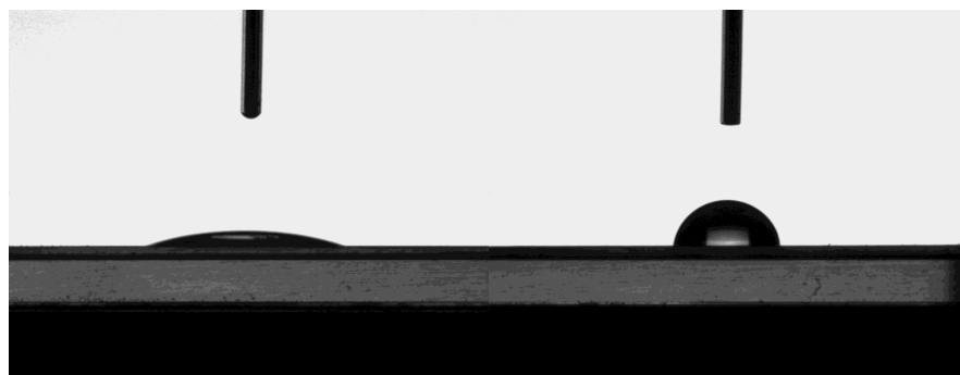
Figure 3-5: Water contact images of (left) pristine PPF ( WCA = 17^\circ \pm 3 ) and (right) Au_{25} -PPF after dipping for 10 minutes in a 1.9 mM solution of [TOA][Au_{25}L_{18}] in acetonitrile ( WCA = 87^\circ \pm 1 ).
